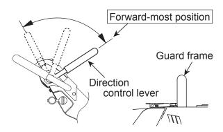
Figure 27. Direction Control Lever (Forward Position)
